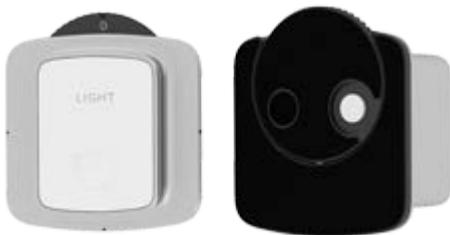
**Zero adjust:** If prompted to make a zero adjust, select zero adjust (0) on the sensor wheel. The zero adjust will take approximately 10 s.
