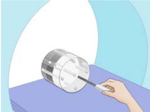
Push the connected sensor tight into the phantom ...
