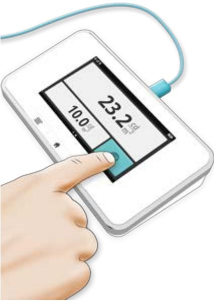
**Tip!** Tap a parameter to get large digits and parameter information. Switch between these by swiping sideways.
