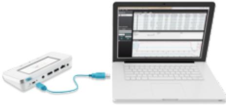
Connect the base unit to a computer running X2 View using a USB cable. X2 View can be installed from the X2 View CD, that came with the system.
