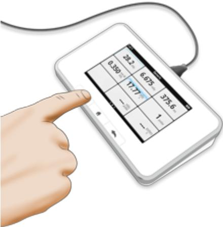
**Tip!** Tap a parameter to get large digits, parameter information, and, if applicable, waveform. Switch between these by swiping sideways.
